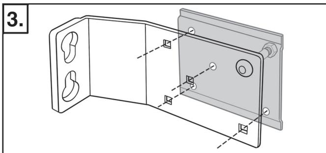
**Important :** To ensure the fit of the backing plates the 3/8" mounting bolt holes must be drilled accurately, perpendicular and straight through the door.
